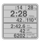
Pace is expressed as time per 500 meters. This is displayed in the central box on the PM (Performance Monitor). A pace of 2:28 means that it takes you 2 minutes and 28 seconds to row 500 meters. The smaller the number, the less time it takes you to row 500 meters. So, the smaller your pace number, the faster you are rowing. NOTE: At the end of a fixed distance piece, your average pace for the piece will be displayed as ave/500m.
